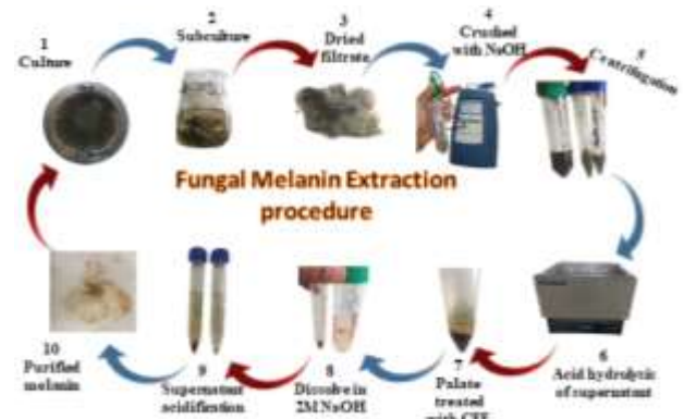
Fig. 2: Step by step mechanism of Melanin extraction from fungus by using acid-alkali method.
